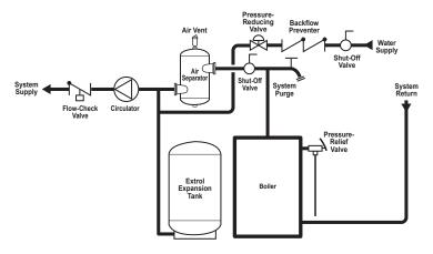
Sizing based on: Average Boiler Water Volume; Average Water Volume; Fill Pressure 12 psig; Relief Pressure 30 psig For other boiler sizes or operating conditions, consult Amtrol Technical Support
