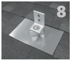
Using a 1/2 inch socket on an impact gun drive the lag screw until the QBlock stops rotating easily. **DO NOT over-torque.**
