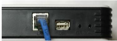
Your DSL/Cable modem plugs into then WAN port of your router/ The Modem plugs into the WAN port of your Ethernet Switch. The existing computers and AM-BR plug into your LAN port of the switch.
