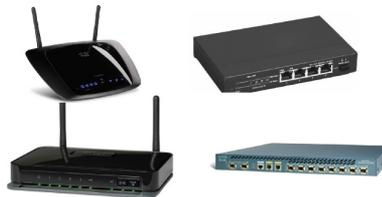
If a modem and a router are both already at the job site, there will be sufficient ports at the back of the router in which to connect AM-BR to the router, with the kit's Cat5 cable.
