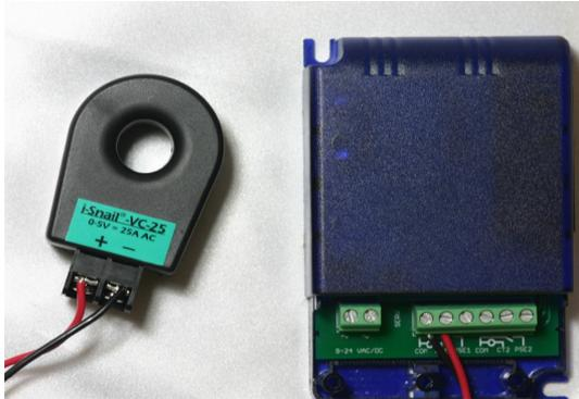
**Run** the live connection to the pump (black or red) through the hole in the CT. While some CTs are directional, that is not the case with this device.
