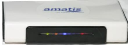
Joule sends AM-BR metered data via IP6 radio. The meter can be installed without cabling between Joule and AM-BR. AM-BR monitors your Internet connection and will store data locally if there is an Internet disruption so the performance data remains coherent.
