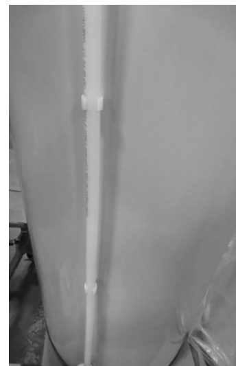
Figure 9 – Installed Sight Glass with Snap Fittings
