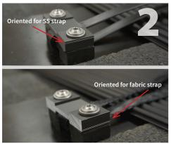
The universal strap cap works with standard stainless steel and woven fabric pool mounting straps. When using the stainless steel strap, orient the cap with the indicator lines upwards. When using the fabric strap orient the cap with the indicator lines downward.
