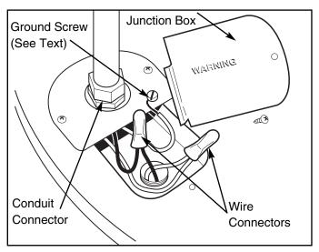
Figure 3. — Water Heater Junction Box.
