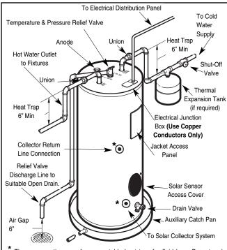
These connections are for non-potable heat transfer fluid loop. Do not make potable water connections to these fittings. Do not introduce non-potable heat transfer fluids into any other tank fitting
