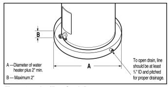
Figure 1. — Auxiliary Catch Pan
