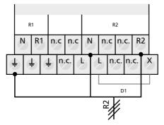
Potential-free output via electromechanical relay; wire bridge must be removed!
