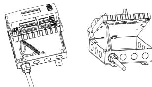
Unscrew the controller from the metal tray before installation. Use a suitable tool to break out the pre-punched holes which are required for the installation.
