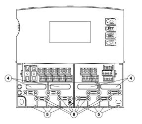
Feeding the cable through the rear of the case:
