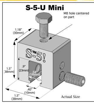
T he S-5-U and S-5-U Mini clamps are each furnished with the hardware shown above. Each box also includes a bit tip for tightening setscrews using an electric screw gun. A structural aluminum attachment clamp, the S-5-U is compatible with most common metal roofing materials excluding copper. All included hardware is stainless steel. Please visit ww.S-5.com for more information including CAD details, metallurgical compatibilities and specifications.
