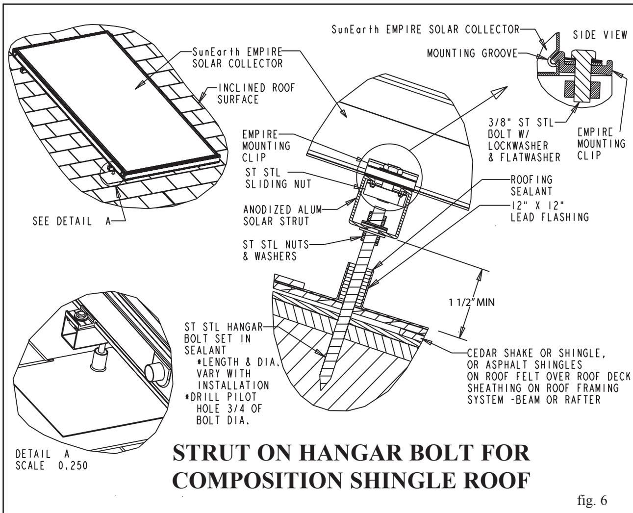
structural members of the roof with stainless steel hanger bolts, lag bolts, standoff mounts or other approved roof attachment method. The solar collector shall be attached to the mounting hardware as detailed in Figures 5–11. (Note: The drawings in this manual detail mounting hardware for the SunEarth Empire series collectors).
