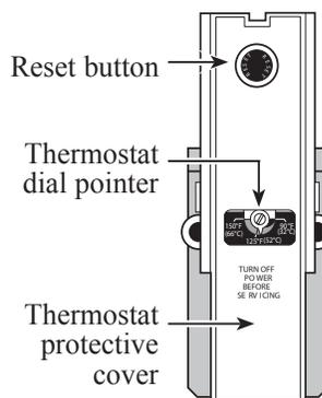
This thermostat controls the water heater's heating element only. (A separate thermostat should be utilized in monitoring the temperature from the collector).
